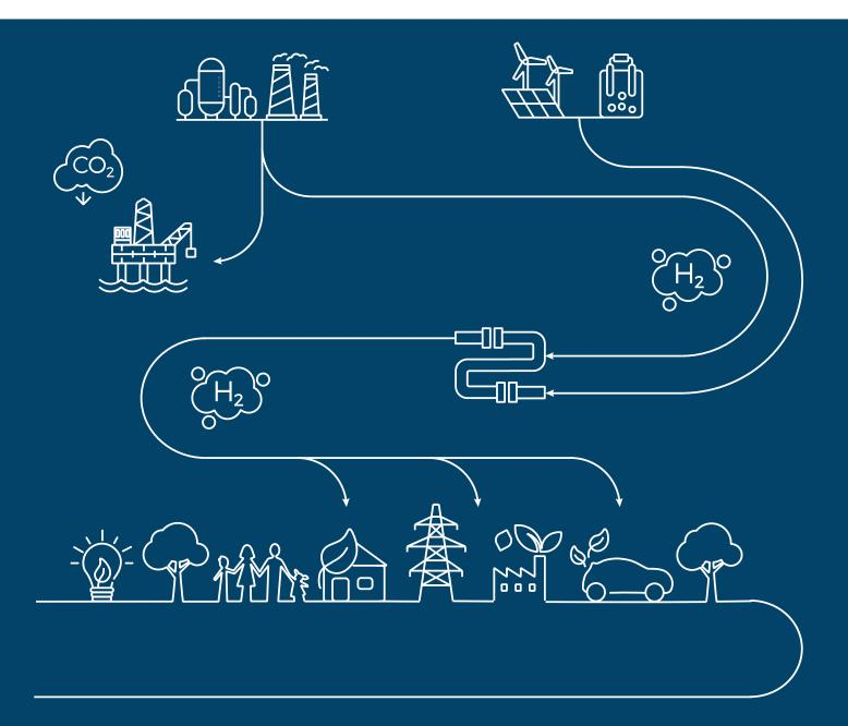
**BLUE HYDROGEN** is produced by 'splitting' natural gas. CO<sub>2</sub> is produced as a by-product of this process, which is then captured and stored underground, offshore. Blue hydrogen is regarded as 'low carbon' because almost all of the CO<sub>2</sub> produced during production never enters the atmosphere.
